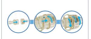
To connect two MPU components, line up and press the two raised features on the insert (or plug) component into the notches on the body (or cap) component, then twist the two components ¼ turn until the two products latch together.
