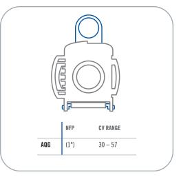
Cv values represent the approximate expected flow rate in gallons per minute of water at room temperature for a 1 PSI pressure drop. The flow is generally constrained by the smallest diameter, which in some cases will be the termination diameter and not the NFP.
