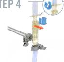
Remove the plastic guard from above the connector thumb latch and transfer it to one of the tabs located directly above it.
