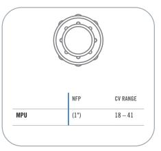
Cv values represent the approximate expected flow rate in gallons per minute of water at room temperature for a 1 PSI pressure drop. The flow is generally constrained by the smallest diameter, which in some cases will be the termination diameter and not the NFP.
