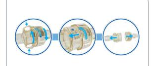
To disconnect two MPU components, depress the two latches on the insert (or plug) component while twisting the two separate MPU components ¼ turn to separate.
