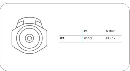
Cv values represent the approximate expected flow rate in gallons per minute of water at room temperature for a 1 PSI pressure drop. The flow is generally constrained by the smallest diameter, which in some cases will be the termination diameter and not the NFP.
