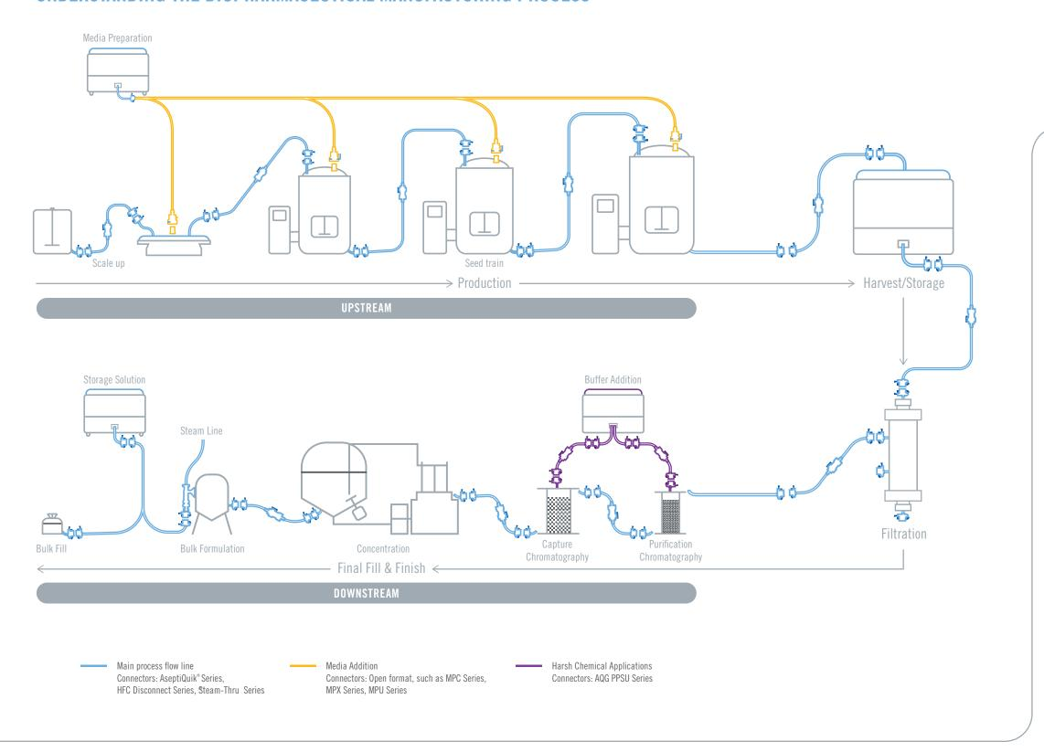
Single-use bioprocessing is designed to be flexible, efficient, and effective in the manufacture of drug substances, monoclonal antibodies, vaccines, biosimilars and regenerative medicines. The process is split into two main sections, upstream and downstream.
